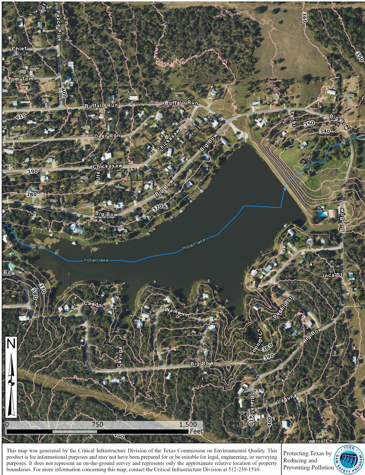
Figure 2 – Aerial View of the Dam with 10-ft Elevation Contours from 2017 LiDAR data & National Hydrographic Dataset Flowlines
